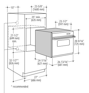
Locate electrical outlet within 10" of left side of opening 34" above cutout floor or 5" below cutout floor.
